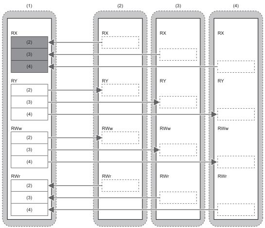
: Area where an input from an error station is cleared
