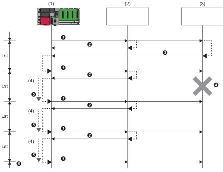
(Slave station disconnection detection setting: Timeout time = 500 ms, number of times = 3 times)
