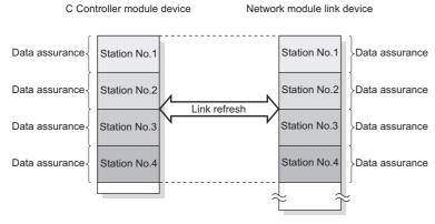
For details of the station-based block data assurance function and the other data assurance functions, refer to the user's manual for each network module.
